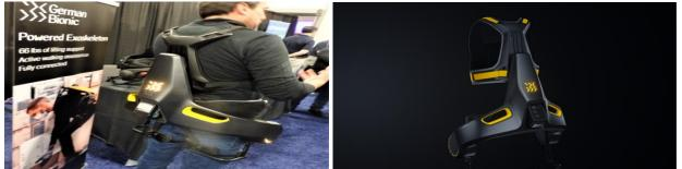
The German Bionic Cray X powered exoskeleton helps to protect the health and wellbeing of those involved in manual handling tasks at the workplace. The Cray X power suit provides up to 66 pounds of support per lifting movement. The suit received a CES<sup>®</sup> 2023 Innovation Award as "Best of Innovation".
