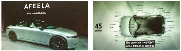
Sony and Honda unveiled the AFEELA, an electric midsized sedan. The EV's entire body comes equipped with 45 cameras and 45 sensors to detect objects and provide an autonomous driving experience.
